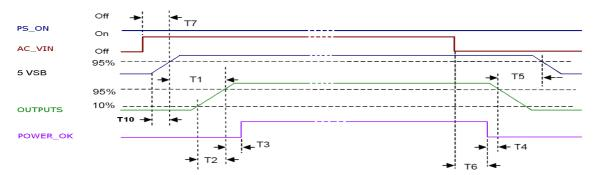
Above waveforms are expected with AC Input ON/OFF:
