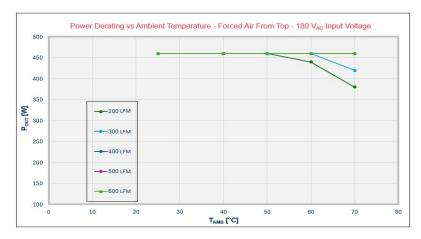
The above curves come from a climatic static chamber and a specific set up therefore they represent a thermal performance approximation of a MDP520 installed into a system where not all the variables can be controlled. Although they are a reasonable reference, it is always a recommended practice to monitor the power supply critical components temperature when operating into a system (see below hot-spots thermal map).
